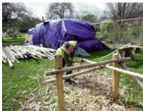
Splitting ash poles using the cleaving brake.
