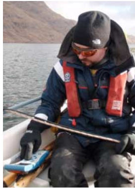
Measuring water quality parameters such as conductivity, temperature, oxygen and pH.
