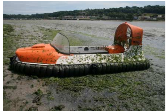
EPA hovercraft, used for safely accessing soft intertidal muddy areas, after a survey of sea lettuce accumulations in Co. Cork.
