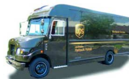
UPS Truck with pilot Hydraulic Hybrid Technology.
