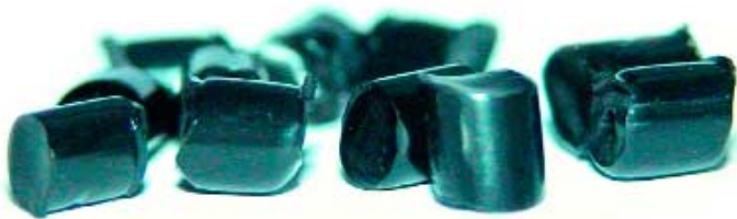
Impact Modified Black Pellets (magnified) which can be moulded into products such as cable ties, nylon wheels, sockets etc...
