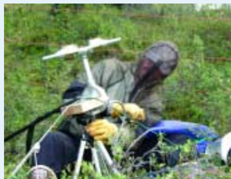
Battling mosquitoes and wary of bears, the WACAP researchers developed portable lab equipment, such as this hand-powered centrifuge, that could be carried to remote locations and operated without auxiliary power.
