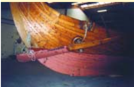
"Starboard": Details of the steering oar of the "Icelander"; during an overhaul.
