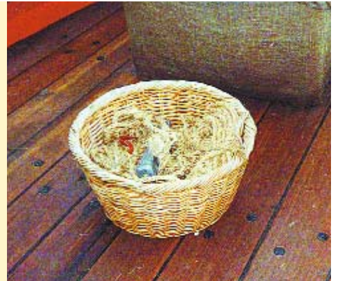
"Swinging the Lead": Lead line for measuring depth of water under ship.
