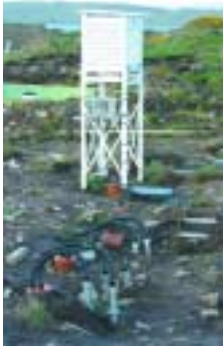
The Stevenson Screen. Note the tubes for the Earth PRT's in the foreground.
