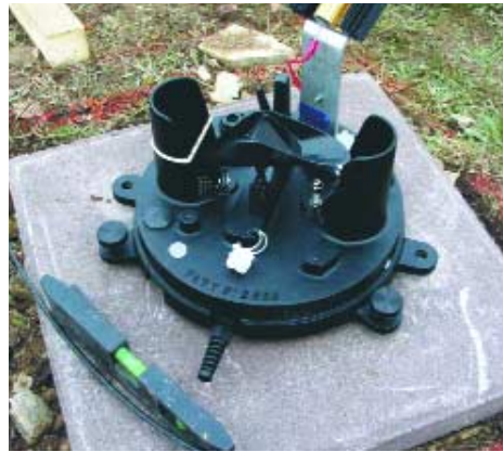
A tipping bucket Rain Gauge. This is the 0.1mm gauge being levelled in its position.
