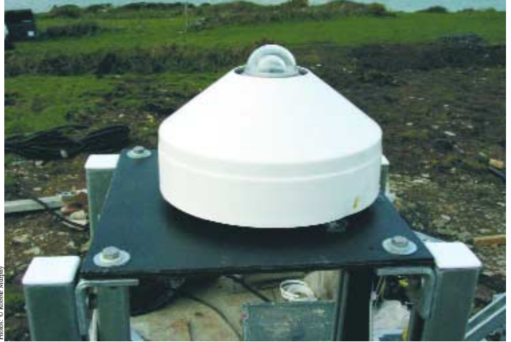
The Solarimeter – for sunshine measurement.
