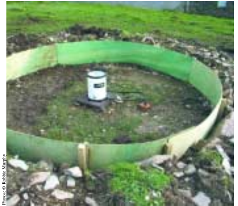
The rain gauge with its turf wall.
