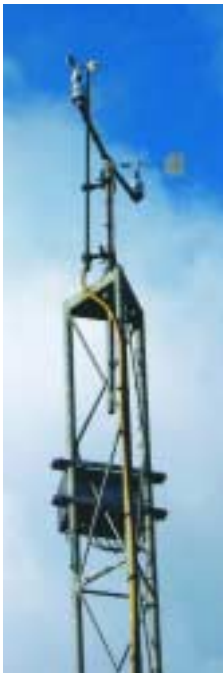
The anemometer sensors at the top of the mast. The crossarm is fitted due N-S with the direction vane on the northern end.
