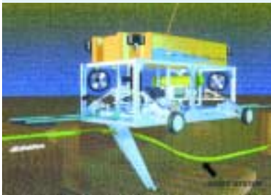
Hydraulic jet fluidises seafloor and cable sinks into bottom.
