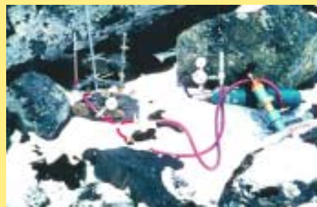
Apparatus for field determination of nitrogen fixation using 15\text{N} as a tracer. Signy Island, January 1966
