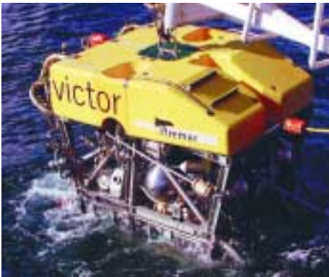
VICTOR is a state-of-the-art remotely operated vehicle which was deployed from the French mother ship ATALANTE.
