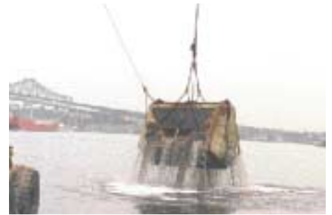
Above left: Deepening harbours can require removing rock. The Dredge "New York" is working beneath the Fitzgerald Bridge in inner Boston Harbour. Top: As cargo vessels increase in size and draft, Ports must deepen channels to remain competitive. Boston has just finished their new 45 foot deep channel. Above right & top right: Different sediment calls for different dredges: the ripper is used in hard soil and soft rock (above right), the clamshell is used in soft and soupy sediments (top right). The power ripper shovel dumps its 10 yard bucket into a disposal scow for transport to a designated dump site. Clamshell dredges can move up to 50 cubic yards in a single grab.
