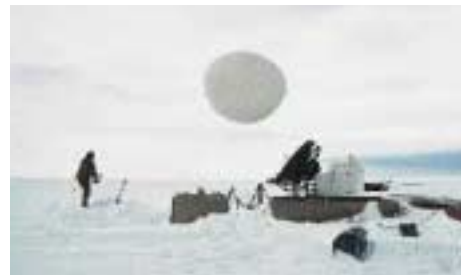
A radiosonde balloon being launched at the British Antarctic Survey's Halley Station. It will be traced by radar and give information about upper air winds.
