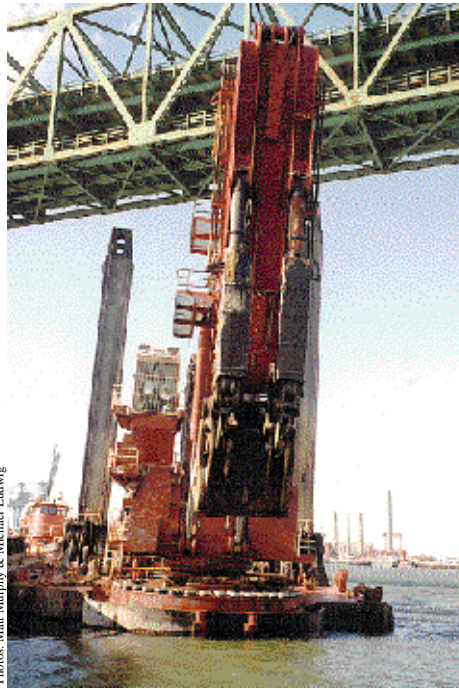
Above left: Deepening harbours can require removing rock. The Dredge "New York" is working beneath the Fitzgerald Bridge in inner Boston Harbour. Top: As cargo vessels increase in size and draft, Ports must deepen channels to remain competitive. Boston has just finished their new 45 foot deep channel. Above right & top right: Different sediment calls for different dredges: the ripper is used in hard soil and soft rock (above right), the clamshell is used in soft and soupy sediments (top right). The power ripper shovel dumps its 10 yard bucket into a disposal scow for transport to a designated dump site. Clamshell dredges can move up to 50 cubic yards in a single grab.
