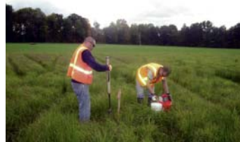
As part of the clean up, the floodplains, low-lying shoreline areas, are also being evaluated for the presence of PCBs. More than 5,000 soil samples have been collected since 2002. These samples are analysed for PCB concentration.
