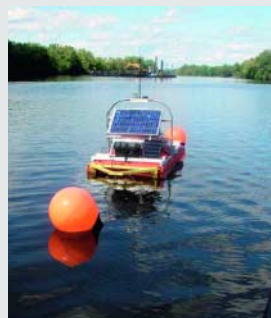
The project’s effect on water quality is closely monitored in accordance with Engineering Performance Standards. Water monitoring is done around and downstream of the dredges, to determine PCB resuspension levels. This water monitoring buoy is solar powered.
