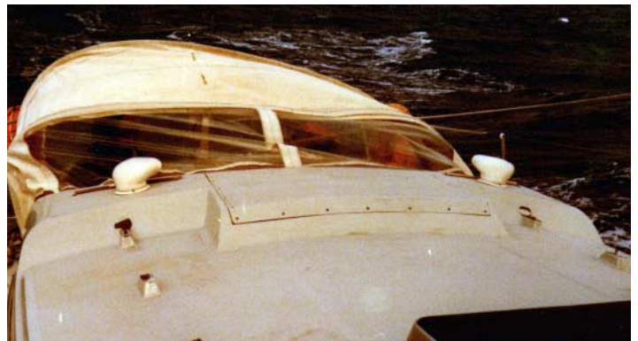
Shardana's spray hood was flattened when the boat went over.
