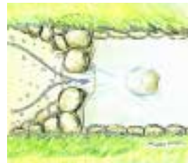
A simple single notched weir is the most suitable stone weir structure for small channels (< 3.5m basewidth). Monitoring data indicate that they have greatly increased the salmonid carrying capacity of small channels for 0+ to 1+ year-old fish.
